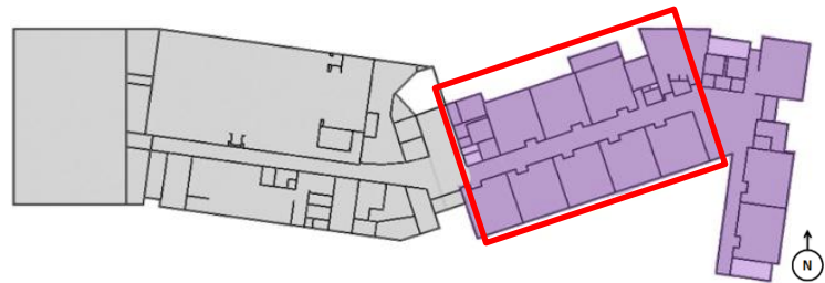
Figure 21: Education Wing Highlighted on Building Floor Plan with Structural Bay Redesign Called out in Red
